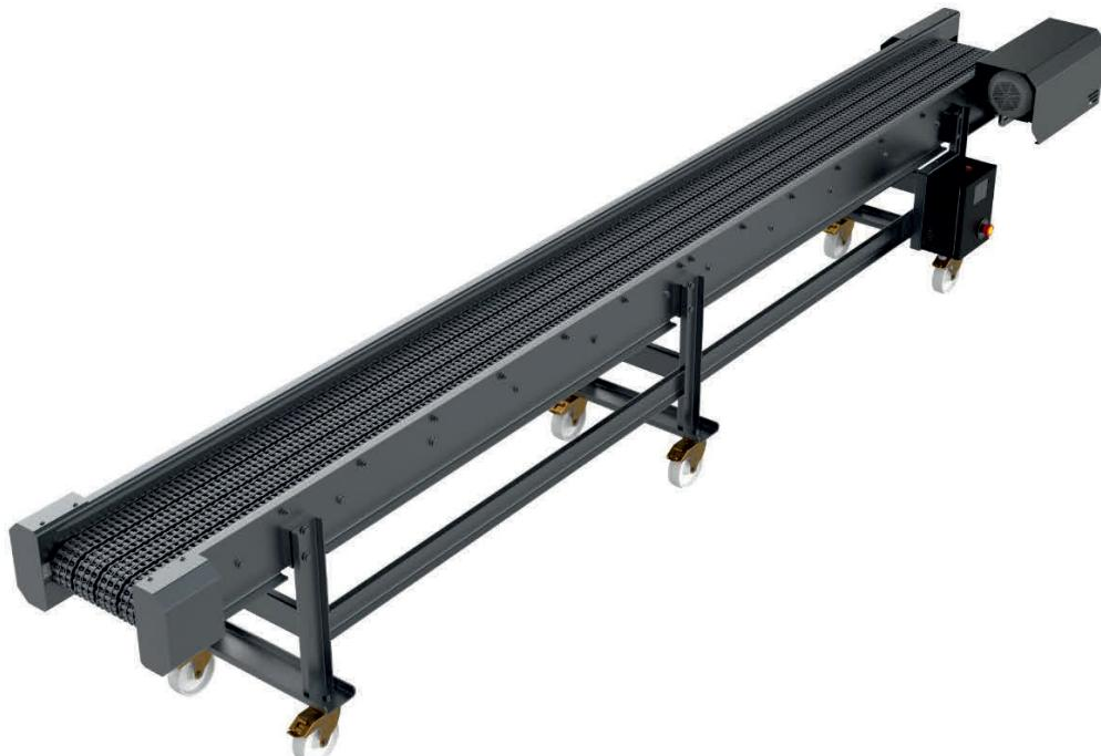
Hot parts transport conveyor is a heavy-duty type of transport system that allows metal billets or pre-forging parts that are treated with high temperatures (usually 900-1250°C) in induction furnaces to be transported to forging press, rolling mill or the next process station without losing their thermal properties and deformation.
