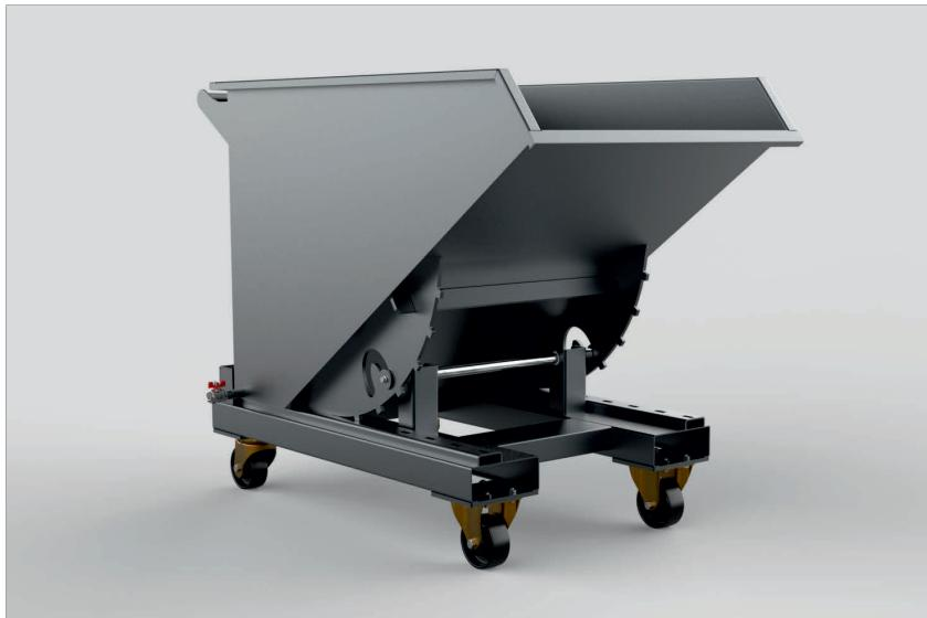
Chip carts are braked and tilting wheeled carts which are used for collecting chips which come from chip conveyors. It can be easily moved under conveyors and emptied to chip storage with its special design. Coolant liquid/Cutting oil, which will be accumulated in the chip cart can be discharged from discharge valve located on the bottom of the cart. It can be manufactured in different sizes and capacities.
