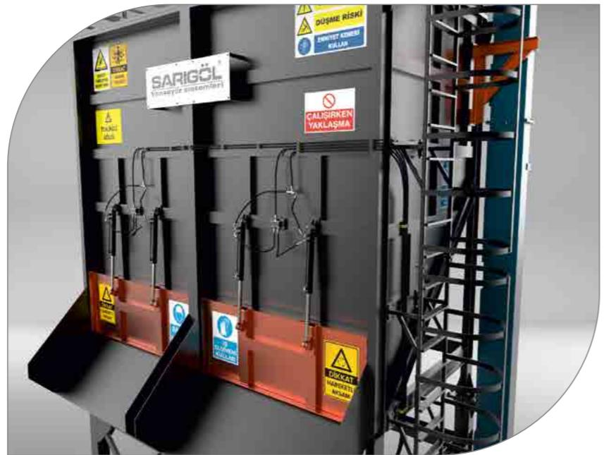
Chip silos are used to store high capacity chips which come from line conveyors and to transfer chips to trucks when required.
