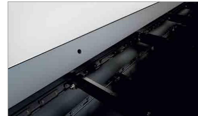
Scrapers conveyors are used to convey small chips and particles which come from grinding and honing various composite materials such as iron, cast-iron, brass-alloys, and sintered metals. These models uses scraping method to take out the particles by rubbing them to the floor. The conveyor can also operate with no coolant (water) with friction safe hardox iron sheets mounted on the floor and in between the belt rails.
