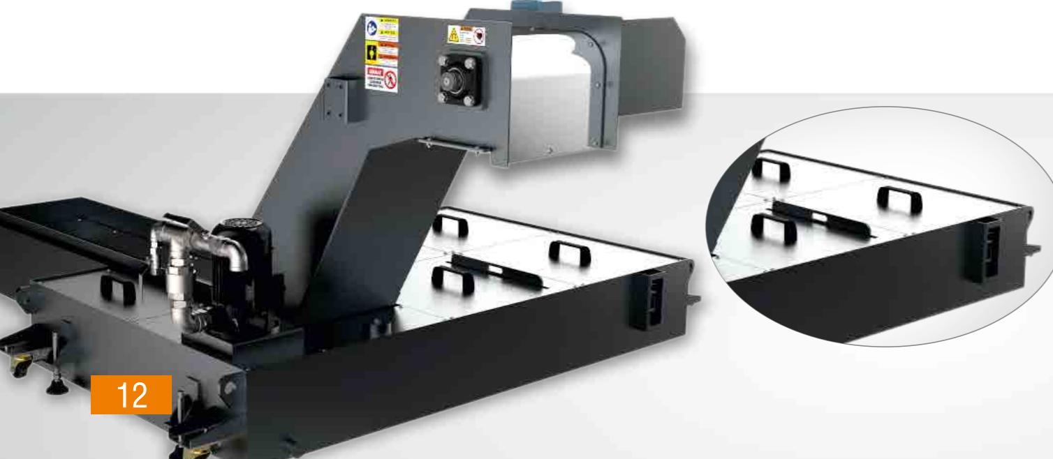
Magnetic conveyors are used to carry dust, crumbed iron chips, and other metal particles. There is no damage risk of pallet and particularly the product carried since the magnetic carriers has no contact product and chips. The production cost of these type of conveyors is the highest due to the neodymium magnet mounted on the pallets.
